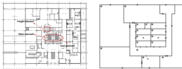
Figure 2. The floor plane of the 1 st floor (left) and corresponding CONTAM model geometry (right).
